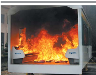
Fig. 1 Fire test in a mock-up train(KORAIL)
