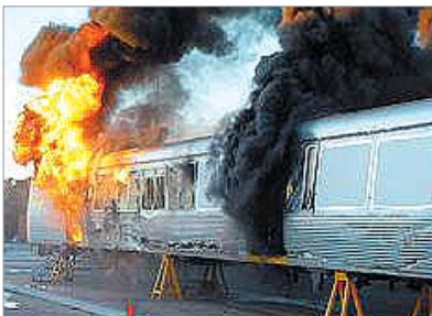
Fig. 2 Fire spreads in 3 minutes after ignition(CSIRO)
